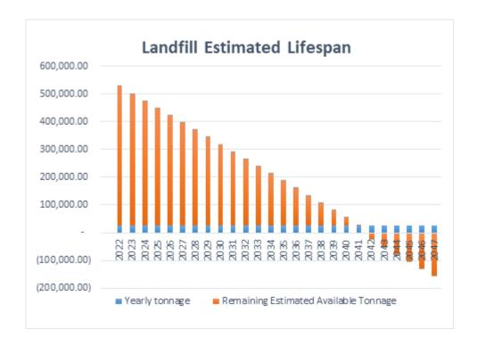
The average tonnage received at the City of Kenora landfill for the past ten years has been calculated to be approximately 26,228 tons per year. As indicated in the Landfill Estimated Lifespan chart, the landfill is expected to reach its designed capacity by 2041. Should the City continue to encounter volumes in excess of 26,228 tonnes per year, the lifespan of the facility will continue to erode and require replacement sooner than 2041.
